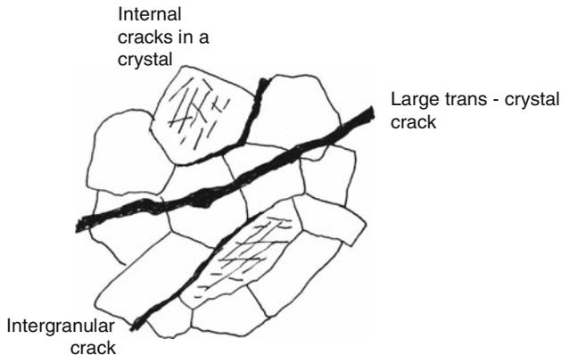
**Fig. 2.2** Different types of cracks and fractures common in rocks due to their thermal and tectonic history. (1) Internal fractures within a crystal (2) inter granular fractures (3) trans-crystal fractures. All lead to the introduction of water into the different passageways in the alteration process of water – rock contact at the surface
