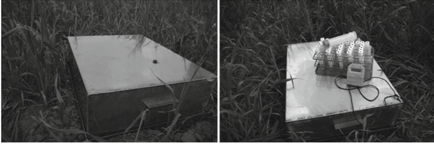
**Fig. 5.1** Closed chamber for in situ emission measurements
