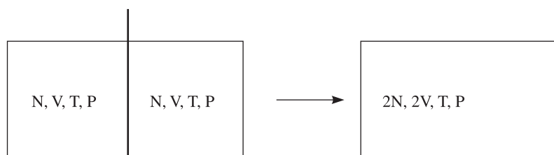
Fig. 6.4.2 Mixing of two identical samples of the same gases
