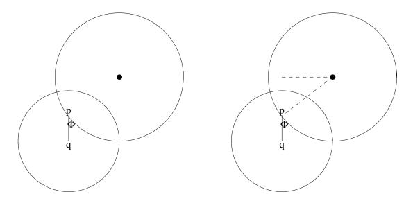
Draw the two additional dotted lines indicated on the right, and notice that these lines meet at an angle  $\Phi$  because each dotted line is perpendicular to a side of the original angle  $\Phi$ . The side opposite this new angle is the radius of the large circle minus the Euclidean distance from q to p. If this Euclidean distance is called r, then
