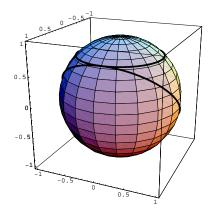
Apply the Gauss-Bonnet theorem to the cap at the top of the sphere. All exterior angles are zero, so
