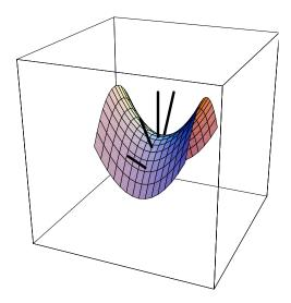
Repeat this argument, but this time move in the y direction, as in the left picture on the following page. (To avoid interference, the normal vectors have been drawn shorter than they should be.) Notice that the change of the normal vectors is now in the negative y-direction. For a standard saddle, we will later calculate that the derivative of n in the direction  $e_2$  is  $-2e_2$ .
