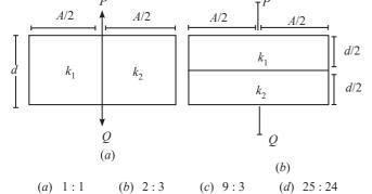
**201.** Three different dielectrics are filled in a parallel plate capacitor as shown. What should be the dielectric constant of a material, which when fully filled between the plates produces same capacitance?
